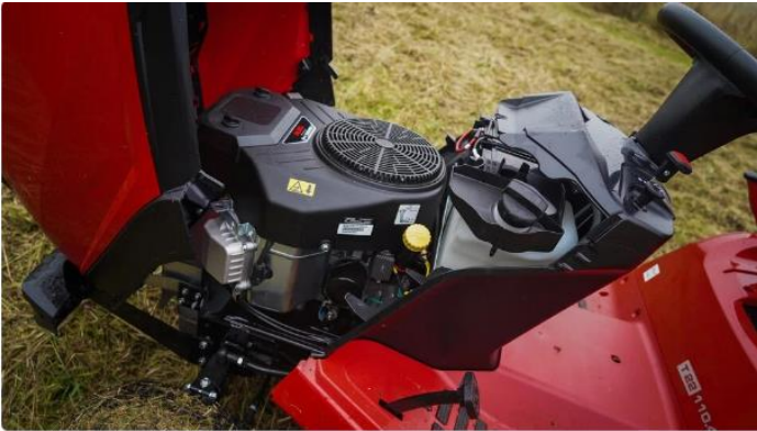
The two-cylinder petrol engine produces 13.KW (18HP). Photo: Jørgen Ahler.
