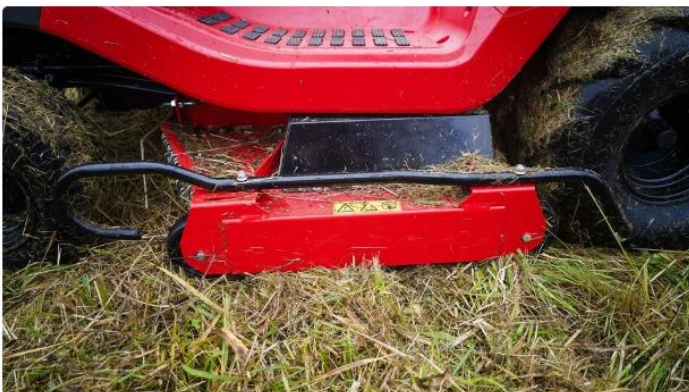
Drive belts and blades are well protected. Photo: Jørgen Ahler.
