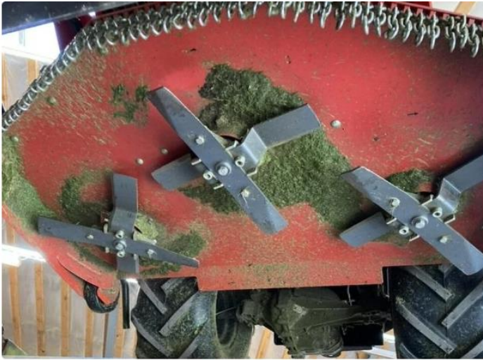
Three powerful cross-cutting blades take care of the long grass. Private photo.
